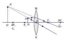
• For magnified inverted image – object between F and 2F of a convex lens
